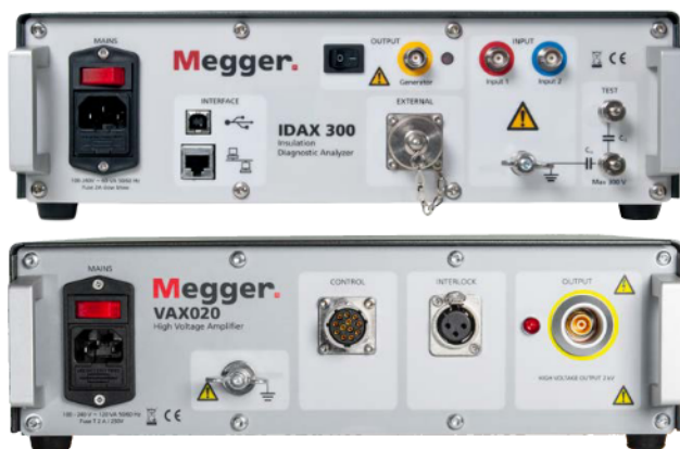
The test system: IDAX-300 and VAX020
